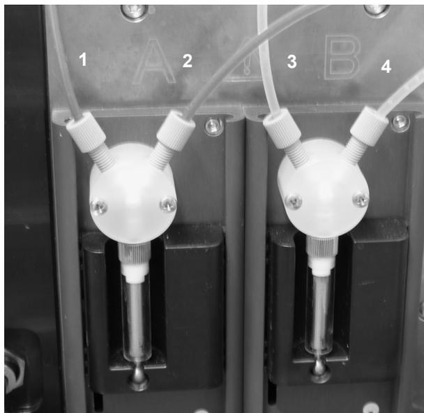
Fig. 16: Mounted hoses of the titration unit
