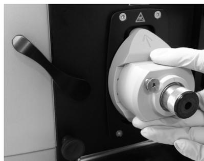
Fig. 55: Take off the measuring cell
