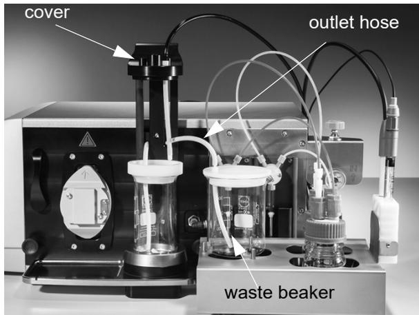
Fig. 56: System configuration while cleaning the system
