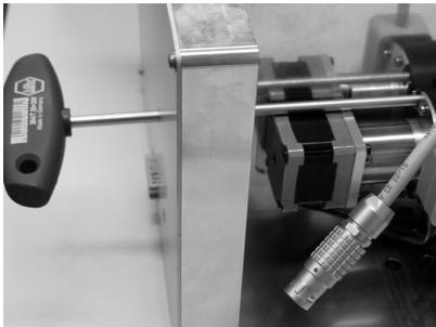
Fig. 13: Loosen the screws of the hydraulic valve motor
