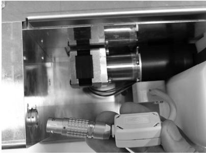
Fig. 12: Connecting the hydraulic valve motor
