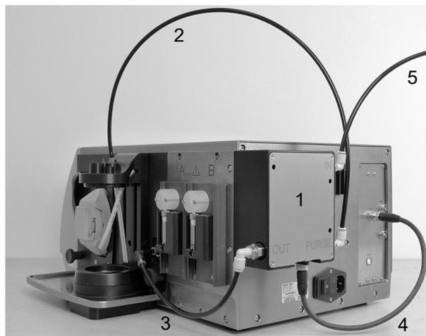
Fig. 18: SurPASS 3 external pressure control
