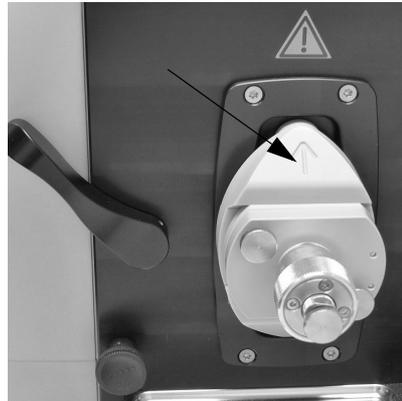
Fig. 41: Arrow on the measuring cell pointing upwards
