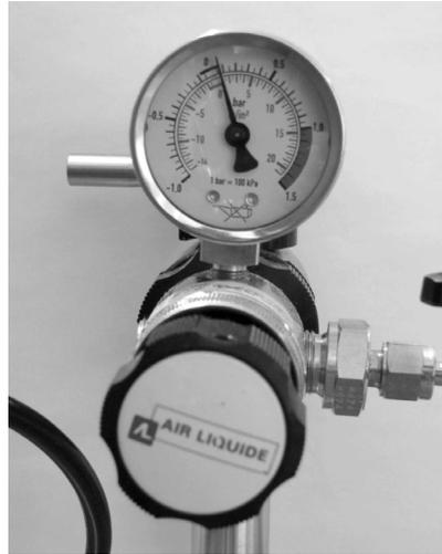
*Fig. C-1: Air Liquide pressure-reducing valve BS 20-1-2 with a resolution of 0.05 bar for use with a nitrogen supply with 20 bar primary pressure.*
