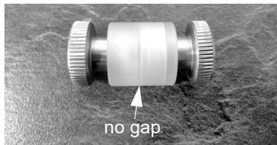
Fig. 35: Closed sample holder with mounting tools
