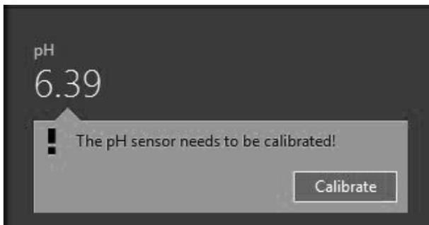
Fig. 20: pH calibration reminder
