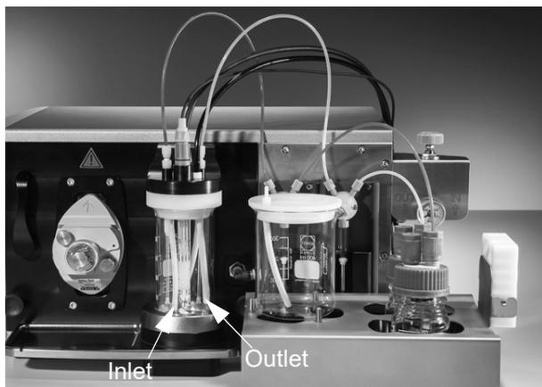
Fig. 53: System configuration while emptying the system
