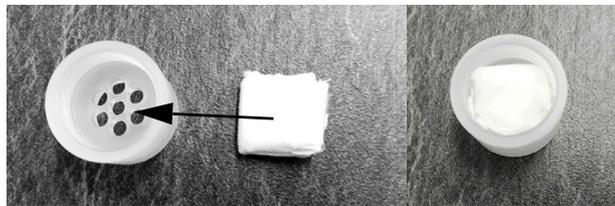
Fig. 34: Mounting the cotton fabric
